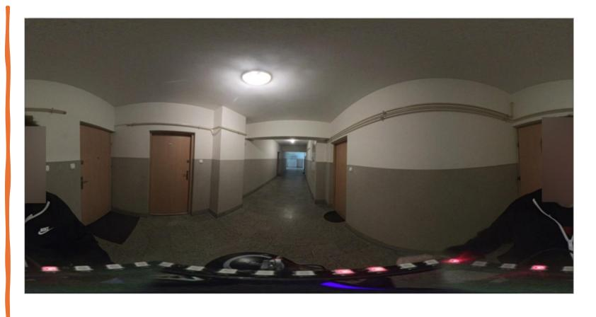
The LED diode ring enables encoding of the timestamp using Gray code, allowing synchronization of the LiDAR and camera with a resolution of 100 ms.
