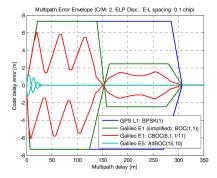
Steeper main peak of ACF relates to lower tracking noise. Secondary peaks improve multipath robustness
