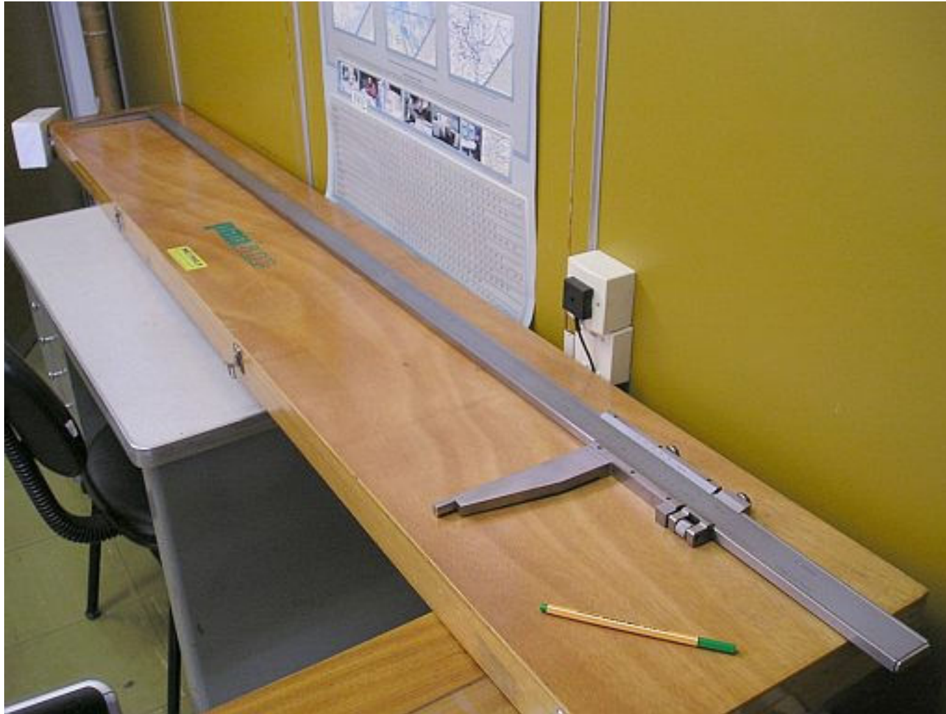
Precision calliper: PANTEC 2000mm / 80", Reading \pm 0,020\text{mm}
